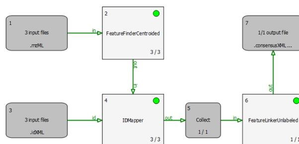
Identifications are mapped to features by the IDMapper. The last step is performed by FeatureLinkerUnlabeled which links corresponding features. The results can be used to calculate ratios, for example. The data could also be exported to a text based format using the TextExporter for further processing (e.g., in Microsoft Excel).
