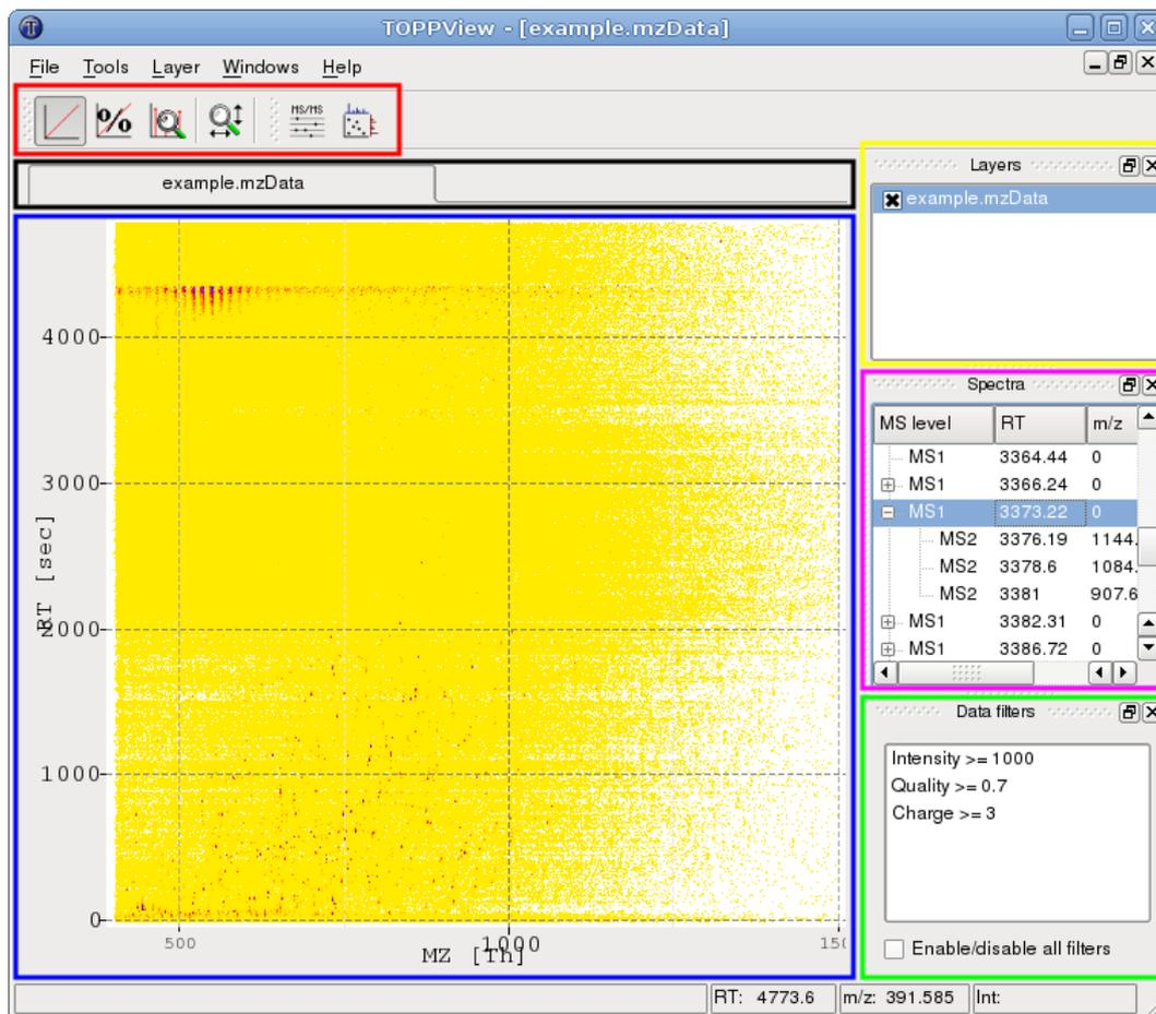
The above example image shows a 2D view of TOPPView (blue rectangle) and the corresponding [Display modes and view options](#) (red rectangle). In the right dock area, you can see the [Layers](#) (yellow rectangle), the [Spectrum browser](#) (magenta rectangle) and the [Data filtering](#) tool (green rectangle). Switching between open windows can be done using the tab bar (black rectangle).
