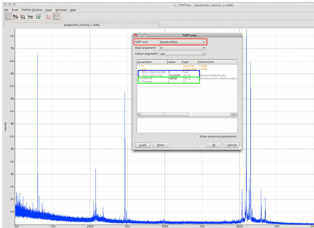
The following image shows a part of the spectrum after baseline filtering as green line, the original raw data is shown by the blue line.
