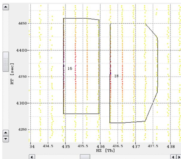
In addition to the normal top-down view, the 2D view can display the projections of the data to the  $m/z$  and RT axis. This feature is mainly used to assess the quality of a feature without opening the data region in 3D view.
